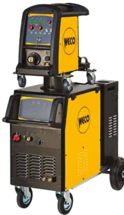
**Pioneer 321MSR - 401MSR** is a synergic 3 Phase Inverter with separated wire-feeder.
